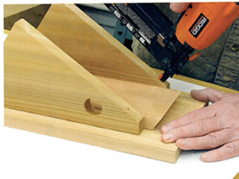
FIGURE 1 Apply glue along the rear edges of the sides and drive a nail through each end to secure them to the back.
