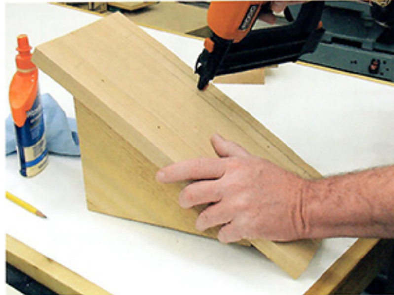
FIGURE 2 Use a pencil to outline where the sides make contact on the other side to use as a guide for nailing.
