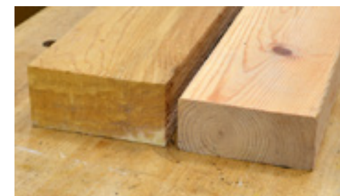
Cedar width and thickness is typically a bit larger than comparable dimensional lumber. The rough cedar 2x4 shown here measures 1\frac{3}{4}'' thick.
