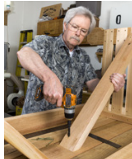
Finish up the table assembly with a pair of diagonal braces. Attach these underneath the table with 3" exterior grade screws.
