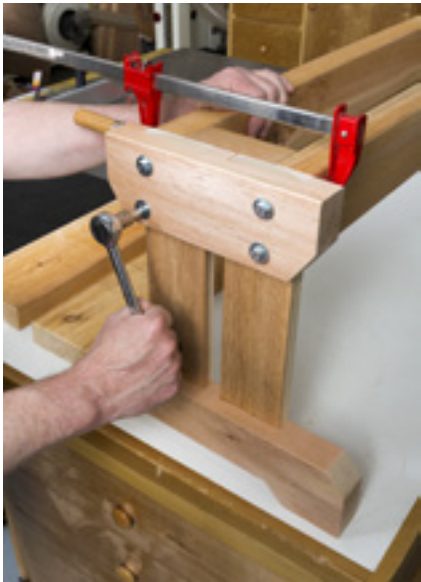
Drill a pair of 1/4" pilot holes for each stretcher through the bench and table ends, then drive home 4 1/2" lag bolts for a solid frame.
