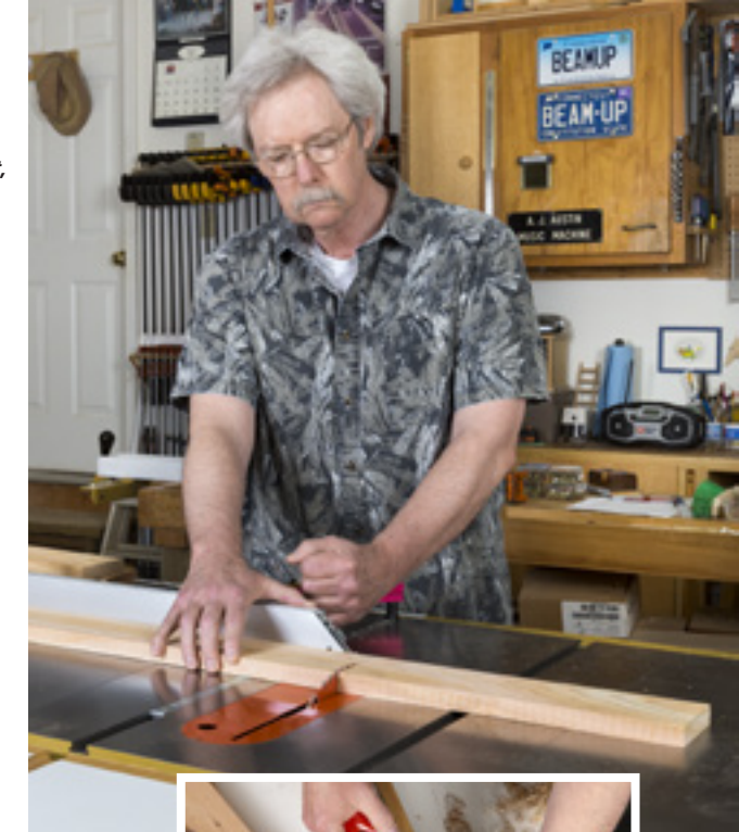
Cut table components to size per the Cut List, but keep in mind any variances in cedar width and thickness.
