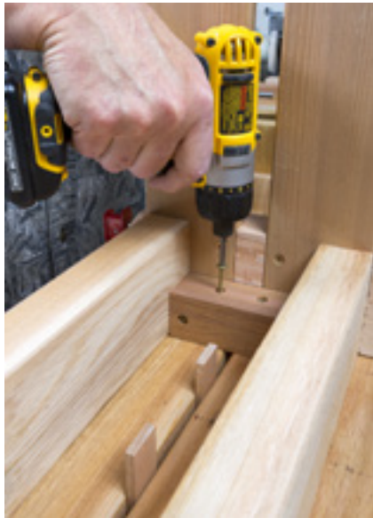
Upend the bench and table frames onto the 2x6 top boards, and drive 3" screws through the cleats to hold them in place.
