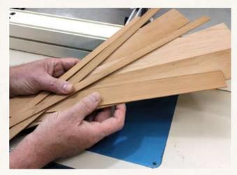
head like shrapnel. Danger aside, the results of planing that thin aren't always optimal. While the box lid and bottom inserts are of thicknesses easily milled in the shop, it's best to purchase bending stock from a woodworking supplier.
