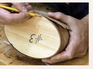
the band off the form to tack it, and will need these marks as a guide to reforming the circular shape on the anvil. When you have the band marked, take it off the form. Now that the wood has cooled, you'll notice that although it pops right out of its oval shape that it's still plenty bent.
