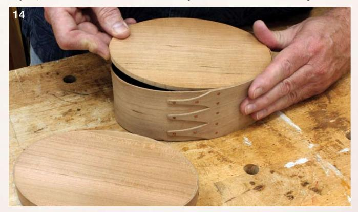
box, I usually space the holes every 2" to  $2^{1}/2$ "; for larger boxes a wider spacing is acceptable. These holes don't need to be deep. Again, for a #3 box a depth of  $\frac{3}{8}$ " to  $\frac{1}{2}$ " is fine.
