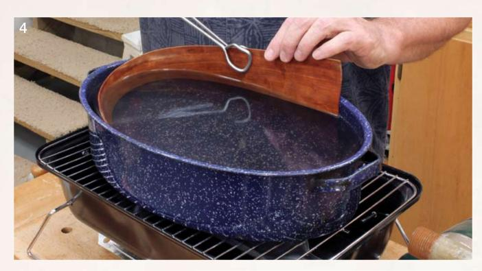
With the two bands prepared, it's time to start "cooking." If you're using a long tray you can just drop the bands in. I'm using a large roasting pan, and in Fig. 4, you can see how I've softened the first portions of the band a bit, then curled it so it can slip into the water around the circumference of the pan. Let the bands soak for 10 to 20 minutes in the hot water.
