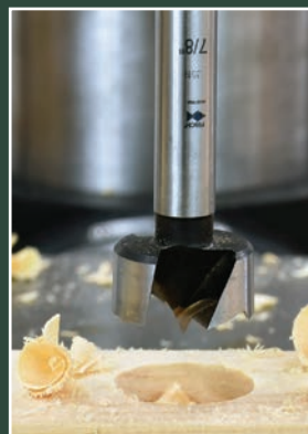
Forstner Bit Cuts large, very smooth and clean holes; excellent for cutting mortises and dowel joinery. Sizes 1/4" to 3 1/2".
