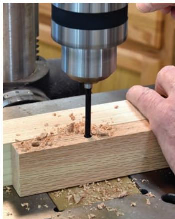
Establish the length of your mortise with a hole at each end inside your stop lines, then remove the remaining waste along the middle with a series of sequential holes.
