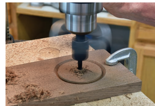
Utmost caution is essential when using fly cutters — you can barely even see it when it’s in motion, but there’s a lot of spinning metal there. Use clamps and keeps your hands well away!
