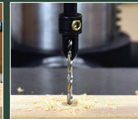
Countersink Bit Variations with or without pilot bit, creates countersink or counter bore to lower screwheads below the material surface. Sizes: Typically correspond to common screw/bolt heads.
