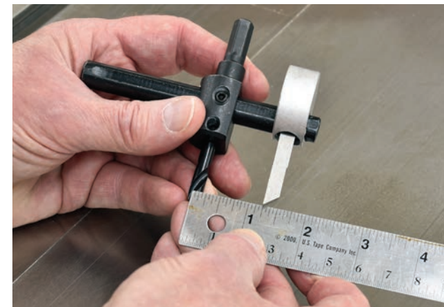
Adjustable circle cutters are set by positioning the tip of the cutter to the radius of the desired hole or disc. Here, a setting of 1/4” will produce a 2 1/2” disc.
