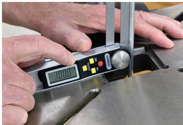
A bevel gauge, like this digital model, helps set table angle in combination with a calibration rod. Originally set at 90 degrees, the bevel now indicates 100 degrees, just right for a 10-degree hole.
