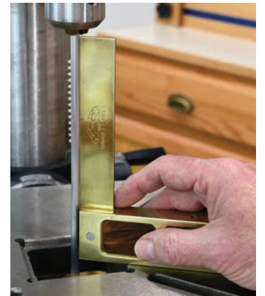
A good accessory to keep with your drill press is a metal calibration rod. Chucked up into the machine, you can use it to check and set precise drilling angles.
