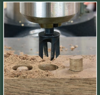
Plug Cutter A hole cutter that excels at creating face-grain plugs; used in tandem with countersunk screws. Both tapered and straight versions are available. Sizes: 1/4" to 1/2".
